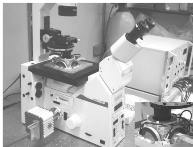
Fig. 6. 3-D MTC device. Close-up of the microscope insert with the temperature control tubing on the right corner is shown at lower right corner of the photograph.
