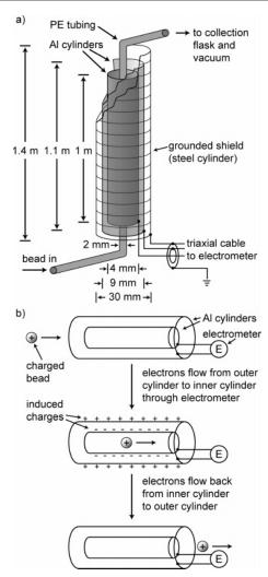
**Figure 2.** (a) Schematic illustration of the apparatus used for measuring the charge on individual microspheres; (b) schematic of the process by which the apparatus measures the charge on a microsphere.
