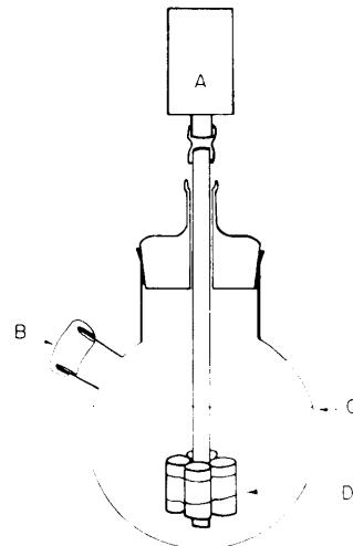
**Figure 3.** Apparatus for following the reaction of a single organic halide with a large excess of magnesium. (A) High-torque, adjustable speed stirrer. (B) Sampling and inert gas inlet through a No-air stopper. (C) Level of reaction solvent (typically ca. 300 mL). (D) Four (originally) 1.00 × 0.625 in. reagent grade (99.9%) magnesium rods bound to the central stirring rod by two pieces of 18-gauge stainless steel wire.
