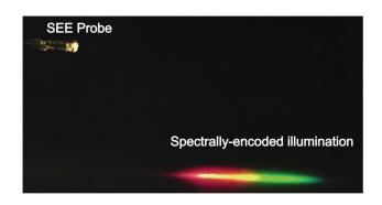
Fig. 3 Photo of the SEE probe and spectrally-encoded illumination.
