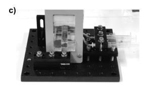
**Figure S3.** Isolating crystal polymorphs. (i) A syringe is used to withdraw the paramagnetic medium and the more dense population of crystals suspended within. (ii) As the first population of crystals from the paramagnetic medium is being removed, the less dense moves with the meniscus toward the bottom of the cuvette. The syringes were disconnected from the tubes and the contents were ejected into an empty container.
