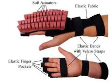
Fig. 10. Top and bottom views of the prototype showing the soft actuators and the open palm glove configuration with the Velcro straps.
