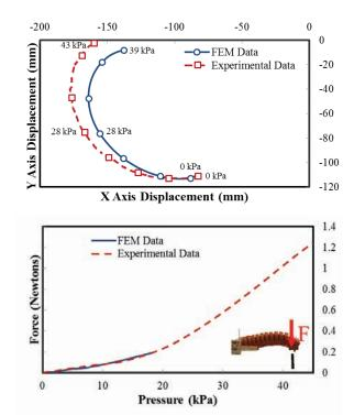
Fig. 9. Top: Comparison of FEM bending curvature and experimental data of the middle finger actuator. Bottom: Comparison of forces for FEM data and experimental data of the middle finger actuator.
