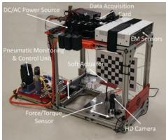
Fig. 7. Photograph of the developed soft actuators characterization platform showing all the individual hardware components.
