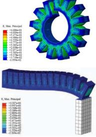
Fig 5. Top: Bending shape response for the FEM actuator. Bottom: Contact interaction shape response for the FEM model. The maximum strain is shown in the legends.
