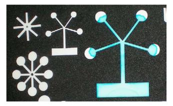
**Figure 3.** The paper devices used in this activity are partially based on these multibranched, lateral-flow devices that do not require patterning to channel liquids to assay areas at the tips of the arms.
