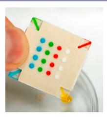
**Figure 1.** Example of a test paper-based diagnostic device from the lab of George Whitesides. This device can conduct four separate tests on four separate samples. Hydrophobically defined channels are made with photoresist (SU-8).
