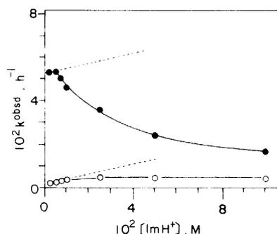
**Figure 5.** Plots of the rates of decomposition of NADH (○) and NADPH (●) against the concentration of imidazolium ion ( $\text{ImH}^+$ ) at pH 7.0, 25 °C. The dotted lines were those anticipated if the magnitude of  $k^{\text{obsd}}$  was a linear function of  $[\text{ImH}^+]$ .
