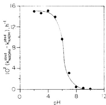
**Figure 4.** Difference between the observed rate constants for decomposition of NADH (0.1 mM) and NADPH (0.1 mM) as a function of pH (25 °C, 50 mM buffer; pH 3.8–5.8, sodium acetate; pH 6.5–8.8, TRA; pH >9, sodium bicarbonate). The solid line was calculated, by using eq 3 with  $pK_a^{\text{NADPH}} = 6.2$ ,  $k_1 = 0.15 \text{ h}^{-1}$ .
