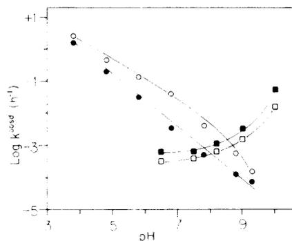
**Figure 6.** Rate constants for decomposition of NADP (■), NADPH (□), NADH (●), and NAD (○) (0.1 mM each) at 25 °C in 50 mM buffer; pH 3.8–5.8, acetate; pH 6.5–8.8, TRA; pH >9, bicarbonate.
