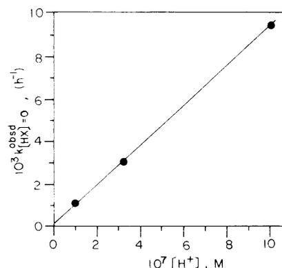
Figure 2. A plot of  $k_{[\text{HX}]=0}^{\text{obsd}}$  (obtained by extrapolating the lines of Figure 1 to  $[\text{P}_i] = 0$ ) vs.  $[\text{H}^+]$  yields slope =  $9.4 \times 10^3 \text{ M}^{-1} \text{ h}^{-1} = k_{\text{H}^+}$  and intercept =  $0.7 \times 10^{-4} \text{ h}^{-1}$  ( $\rightarrow k_{\text{H}_2\text{O}} = 1.26 \times 10^{-6} \text{ M}^{-1} \text{ h}^{-1}$ ).
