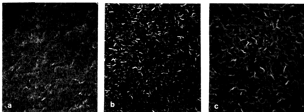
FIGURE 2. Scanning electron micrographs of PE-H (a), and PE-CO 2 H oxidized for 1 min (b) or for 6 min (c) with aqueous chromic acid at 72 C. Reprinted with permission from reference 18. Copyright © 1985 American Chemical Society.
