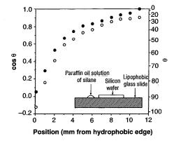
ed from the diffusion of the silane in the vapor phase and subsequent reaction with the surface SiOH groups and adsorbed water on the silicon wafer. The whole assembly was placed in a polystyrene petri dish and covered. The relative humidity of the room was 40% during these experiments.
