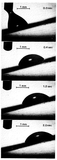
Fig. 3. Uphill motion of a drop of water on a gradient surface. The gradient surface was inclined by ~15° from the horizontal plane. The volume of the drop was ~1 μl. The moving drop was photographed with an automatic camera that exposed one frame every 0.4 s. The drop moved more rapidly on the initial part of the gradient than on the final part.
