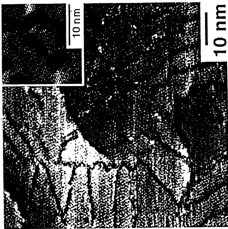
Figure 9 Scanning tunneling microscopy (STM) image of a SAM of dodecanethiolate on Au(111) that shows a gold step, a screw dislocation, and depressed lines in the monolayer due to the accommodation of missing lines of thiols by vicinal molecules. The inset shows five pits in gold that were \approx 0.24 nm deep and linked by domain boundaries. The monolayer packing corresponds to a phase of the c(4 \times 2) rectangular superlattice. These images were provided by Biebuyck and coworkers [62]
