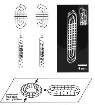
**Figure 12.** A torus. Starting from two mirror-image patterns, we followed the procedure described in Figure 7, and generated a silver torus. The inset figure shows the connection at one end between the two patterns. The diagram at the bottom schematically shows the transformation of a circular torus to a two-cylinder-based torus (in the diagram, we show both tori in a wire form, which are topologically equal).
