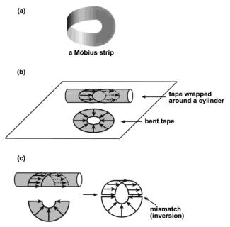
**Figure 2.** (a) A Möbius strip. (b) Schematic illustration of the difference between a strip around a capillary and a strip on a plane. An arrow does not change its direction along the strip around a capillary, which is always along the axis of the capillary, and it does when it moves along the strip on a plane. (c) When joined end to end, the two tapes form a Möbius strip.
