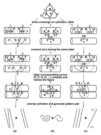
**Figure 4.** Three ways to form patterns that are used to generate trefoil knots. (a) Both "over" and "under" lines of all crossings wind all the way around the cylinders. (b) Neither the "over" nor the "under" line of any crossing winds all the way around the cylinders. (c) Lines of some of the crossings wind all the way around the cylinders. Note that the thin dotted lines are imaginary lines included simply to indicate connectivity.
