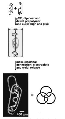
**Figure 11.** Borromean rings fabricated following the procedure in Figure 8. The pattern pair was generated by the procedure described in Figure 4b.
