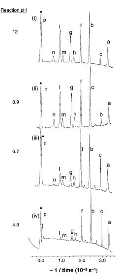
**Figure 2.** Electropherograms (in the 1/time domain) obtained for the reaction of amikacin with 1 equiv of acetic anhydride at different values of pH. Analyses were performed on a Polybrene-coated capillary using 25 mM tris-192 mM Gly (pH 6.9) buffer. Acetic anhydride (530 mM) in dioxane was added to 24 mM amikacin in (i) 60 mM sodium phosphate buffer (pH 12), (ii) 80 mM borate buffer (pH 8.9), (iii) 100 mM sodium phosphate buffer (pH 6.7), and (iv) 200 mM sodium acetate buffer (pH 4.3).
