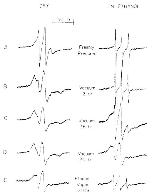
Figure 7. The nitroxyl moieties of PE-CONHNHCSNH-TMPO slowly lose mobility on drying. This immobilization proceeds more slowly if the sample is allowed to stand in contact with saturated ethanol vapor. It is rapidly reversed by immersion in liquid ethanol. Each pair of ESR spectra are of samples treated as indicated after preparation: one spectrum is taken with the film dry in air, the second with the film in ethanol after immersion for 10 min.
