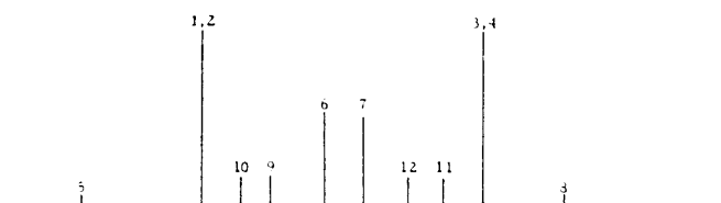
Figure 4. Schematic energy-level diagram and transition assignments for bis(3,3-dimethylbutyl)magnesium.
