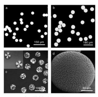
**Figure 4.** Microspheres labeled with a) NBD dye (NBD=4-amino-7-nitrobenzo-2-oxa-1,3-diazole,  $\lambda_{\rm ex}=488$  nm) and b) CdSe quantum dots ( $\lambda_{\rm ex}=502$  nm). c) Polarization microscopy image of 4-cyano-4'-pentyl-biphenyl polyTPGDA microspheres. Inset shows particle morphology at low polymerization rate (see text). d) SEM image of a porous polyTPGDA microsphere.
